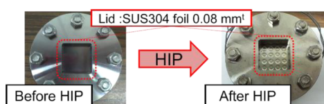
Figure 4. Images of the reaction vessel before and after HIP processing.
